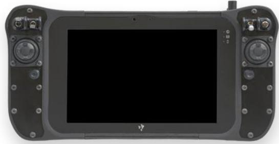
The Micronav is built on top of the Panasonic FZ-M1, a professional and military graded tablet featuring MIL-STD-810G and a 5' Drop and All-weather IP65 Dust and Water-resistant Design. This enables the Micronav to be certified and implemented even in the most restrictive scenarios.
