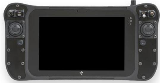
The Micronav Android is built on top of the Panasonic FZ-A2 powered by Android, a professional and military grade tablet featuring MIL-STD-810G and a 5' Drop and All-weather IP65 Dust and Water-resistant Design. This enables the Micronav to be certified and implemented even in the most restrictive scenarios.
